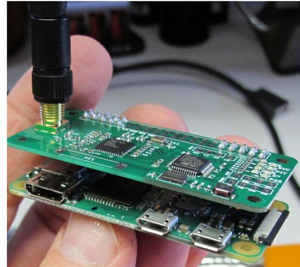
This board provides the RF interface between the Raspberry Pi and your DMR radio.
